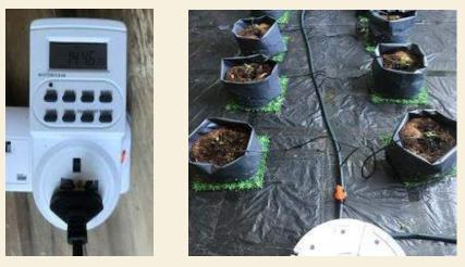
> The fertigation device operates even when the owner is away
